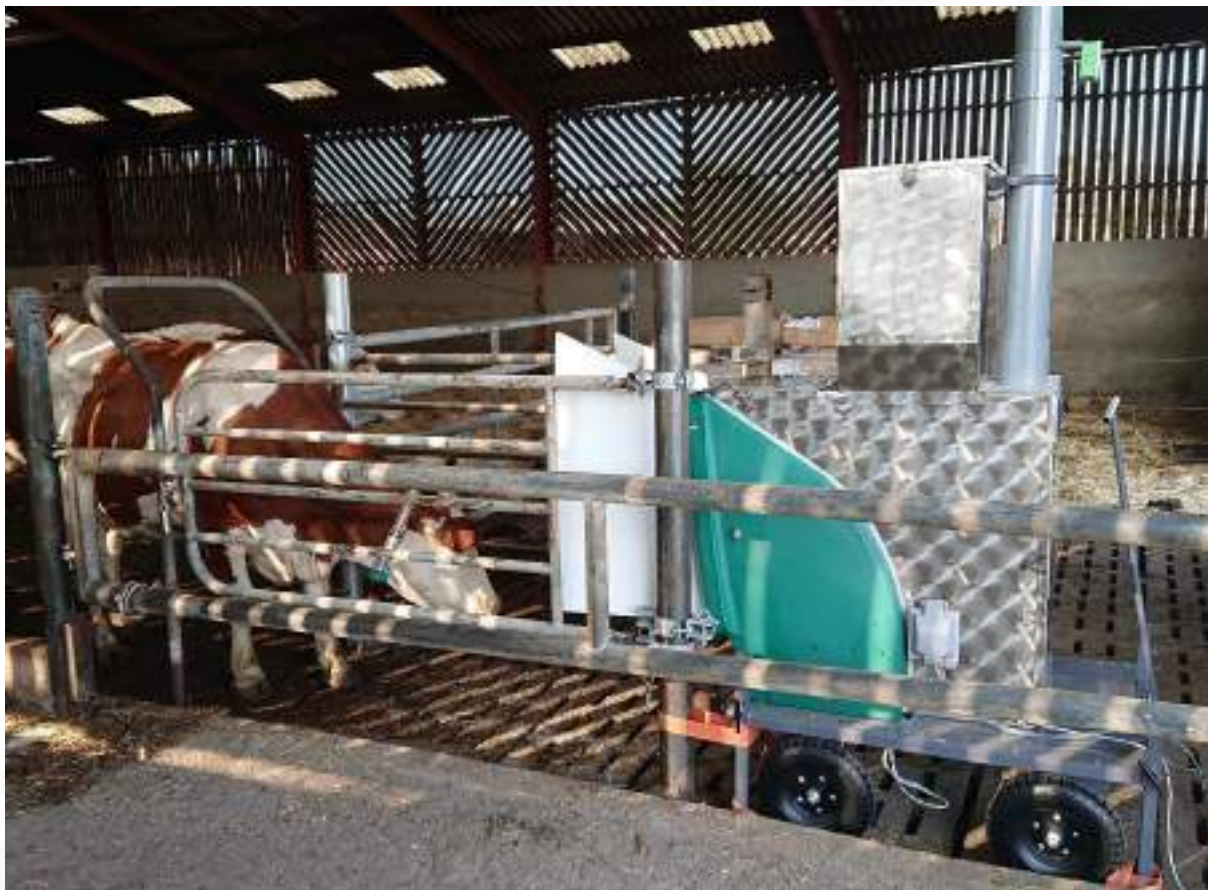
GreenFeed: a tool for measuring enteric methane emissions at individual level
