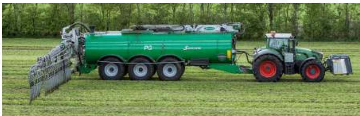
Photo 3. Slurry tanker with equipment for acidifying slurry "in the field" (Henning Foged, enAgro)
