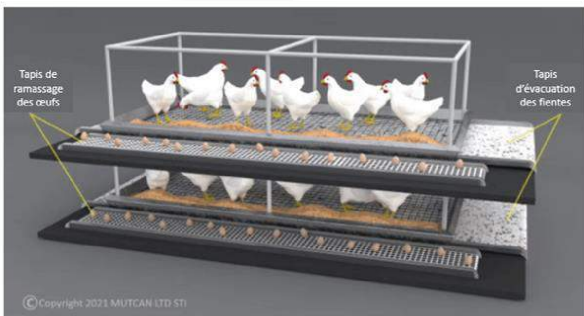
Photo 1: A multi-level poultry cage system with mechanisms for collecting eggs and removing manure efficiently.
