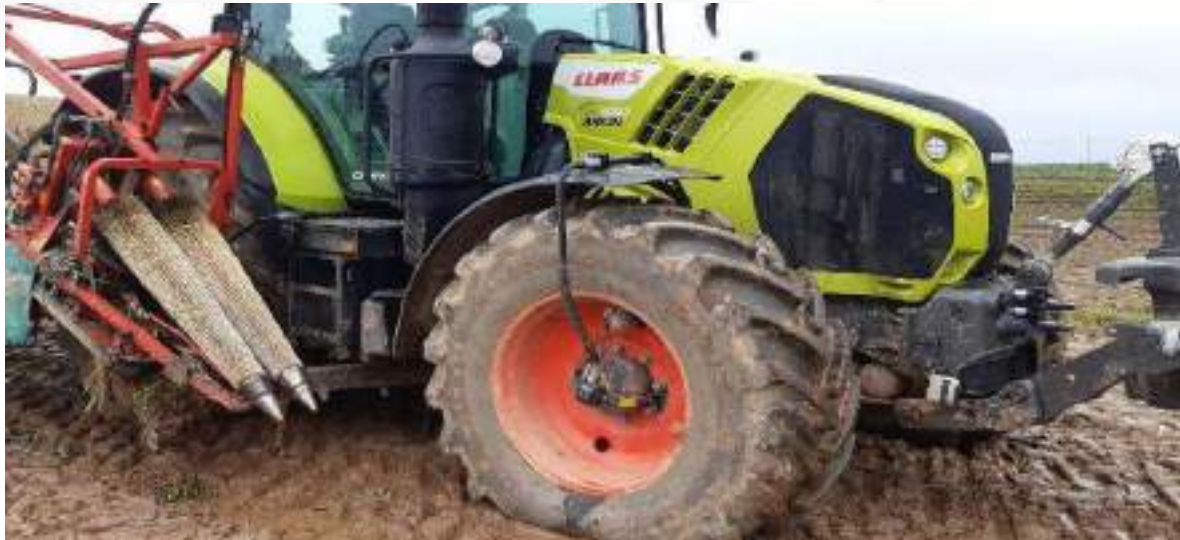
Photo 1: Tractor equipped with a remote tire inflation system to reduce soil compaction
